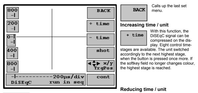
With this function, the DiSEqC signal can be stretched on the display. Eight control time-stages are available. The unit switches accordingly to the next lowest stage, once the button is pressed once more. If the softkey field no longer changes colour, the lowest stage is reached.
